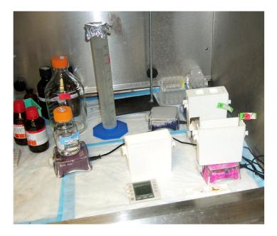
(2) Acetylation is carried out in a white Leica Autostainer container placed on a small magnetic stirrer. The containers accommodate 400ml of freshly diluted 1x TEA (see Stock Solutions for procedure) and a stir bar (25 mm and 5 mm thick). The solution has to be stirred vigorously. When a slide rack is ready after PFA fixation, 1ml of acetic anhydride (Sigma A-6404) is added to the TEA using a repeat Distriman
