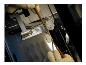
(18) The sections should not be attached to the knife holder block at the edge closer to you (front edge), they might even stick up a little. To pick up the section lower the microscope slide in the slide holder slowly to first catch the front edge of the section. Then slowly lower the slide towards the section that will attach itself to the warm slide.
