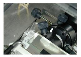
(17) Lift the anti-roll plate carefully. If the anti-roll plate is raised too quickly the section will not stay attached to the edge of the blade. Then take the two small brushes and gently press the edge of the section close to the blade making sure that it attached. If necessary you can straighten the sides of section with the brushes.
