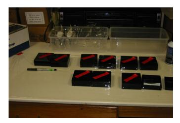
Slide boxes with desiccant bag from Sigma that need to be regenerated in vacuum at 120°C.
