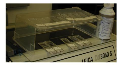
(21) Slides are placed in a slide rack - back to back- with one space in between and are now ready for acetylation. Until a slide rack is full (20 slides), keep it inside the cryostat.
